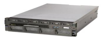
The new S922 has a large memory footprint of up to 4TB and a built-in cloud-optimized hypervisor included at no additional cost
